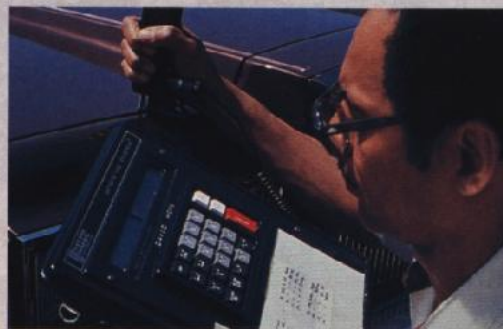
The fit between one body part and the next is evaluated by a computerized measuring device.
