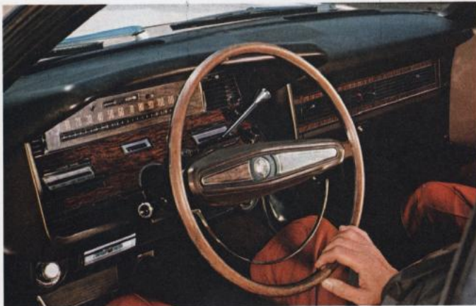
In the pictures on these pages are some of the details as well as the general outlines of the Lincoln Continental for 1968. At the left is a driver's-eye view of the instrument panel, which is almost completely new this year. A rich walnut design sets the tone of the interior. The instruments themselves have been redesigned and there is a new wide-view mirror. The steering wheel has deep padded spokes and hub covered in vinyl, while the upper half echoes the walnut of the panel. The view of the right front of the car reveals the wraparound parking lights, which now are integral with the styling and are a safety feature because they can be seen from the sides. The other two pictures show the lines of the car—in settings appropriate to such automotive distinction
